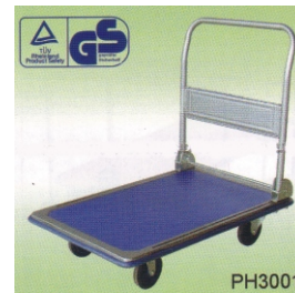
PLATFORM TROLLEY PH 3001 Capacity - 300kg Collapsible handle Size - H850/h195xL907xW608 125 Diameter rubber castors Steel deck with rubber non slip deck and rubber side bumpers
